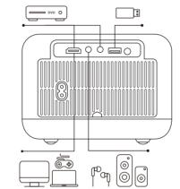
Yaber L1 projector has 4 ports, HDMI port/Headphone Port/AV port/USB port. Please select the correct connecting port to connect your device (PC, Phone, DVD Player, Sound bar, USB, PS4 etc.)
